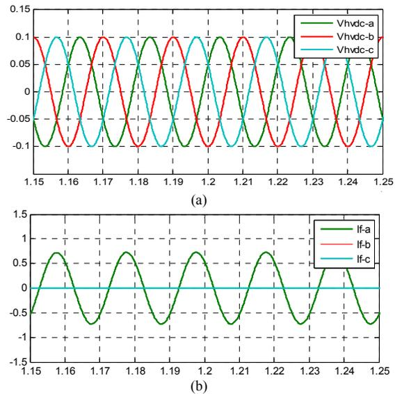
Figure 5. For case i (a) Phase voltages generated by the HVDC [pu] vs. time [s] (b) Fault phase currents [pu] vs. time [s].
