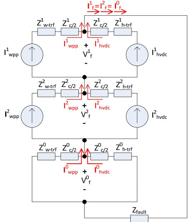
Figure 2. Single-line-to-ground fault equivalent sequence network.
