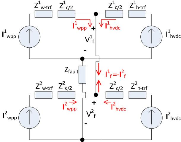
Figure 3. Line-to-line fault equivalent sequence network.
