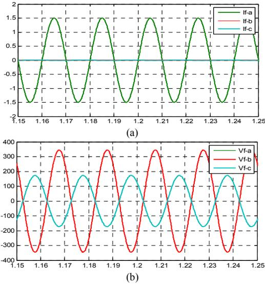
Figure 6. For case ii (a) Fault phase currents [pu] vs. time [s] (b) Fault phase voltages [pu] vs. time [s].
