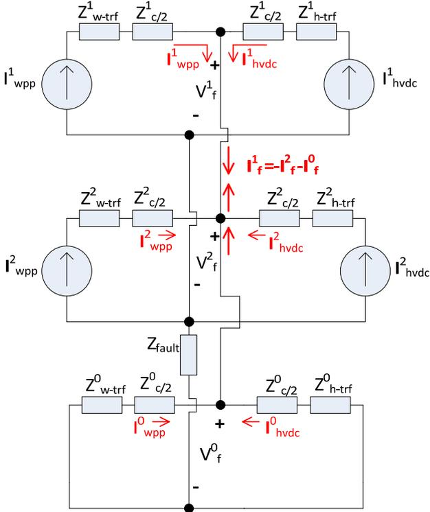
Figure 4. Double-line-to-ground fault equivalent sequence network.
