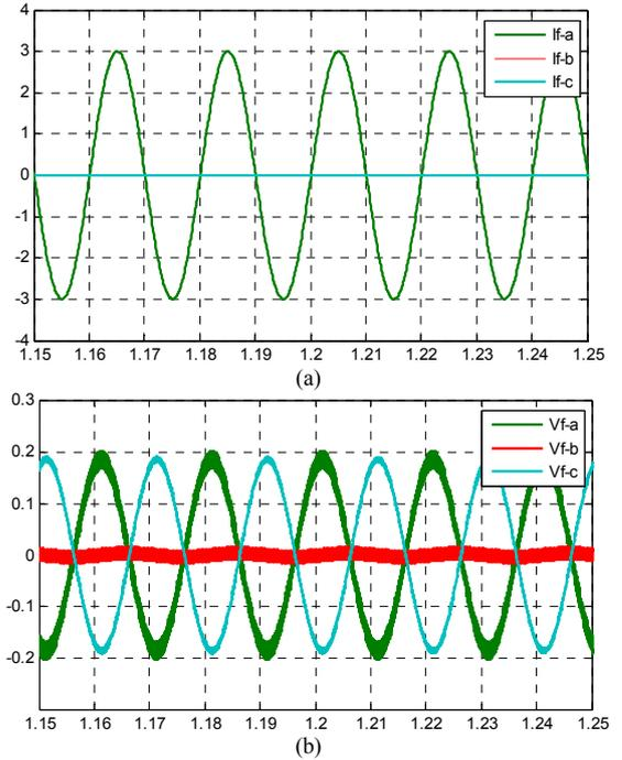
Figure 7. Case iii (a) Fault phase currents [pu] vs. time [s] (b) Fault phase voltages [pu] vs. time [s].
