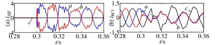
Fig. 10. Differential protection during asymmetrical fault F3: (a) difference of the currents flowing into and out of cable  $Cab_4$  and (b) currents flowing through cluster breaker  $B_{C1}$ .
