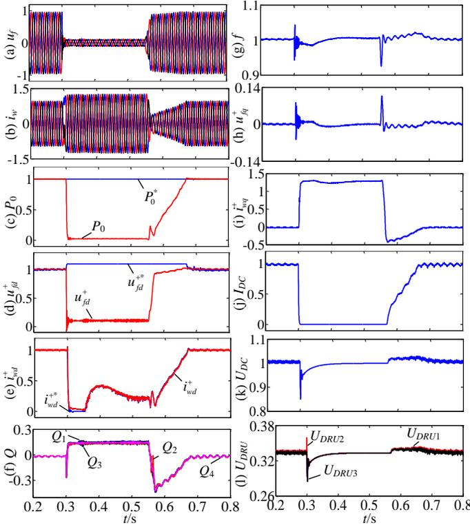
Fig. 4. Simulation results during symmetrical fault F1: (a) three-phase voltages, (b) three-phase currents, (c) active power, (d)  $d$ -axis voltage, (e)  $d$ -axis current, (f) reactive power, (g) frequency, (h)  $q$ -axis voltage, (i)  $q$ -axis current, (j) DRU-HVDC link current, (k) DRU-HVDC link voltage, and (l) DRU voltages.
