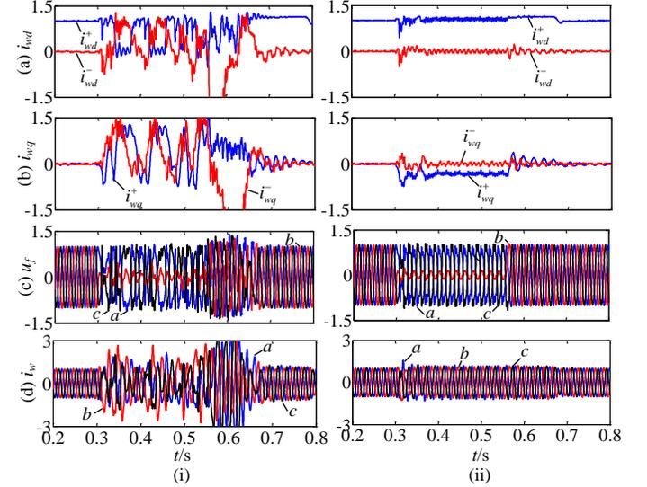
Fig. 5. Simulation results during asymmetrical fault F1 (i) without and (ii) with negative current controller: (a) positive and negative  $d$ -axis currents, (b) positive and negative  $q$ -axis currents, (c) three-phase voltages, and (d) three-phase currents.
