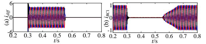
Fig. 9. Differential protection during symmetrical fault F3: (a) difference of the currents flowing into and out of cable  $Cab_4$  and (b) currents flowing through cluster breaker  $B_{C1}$ .
