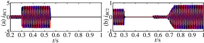
Fig. 7. Three phase currents flowing through circuit breakers during symmetrical cluster cable fault F2: (a) breaker  $B_{C1}$  on the faulty cable and (b) breaker  $B_{C2}$  on the healthy cable.
