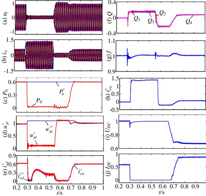
Fig. 6. Waveforms of reduced DC voltage operation during symmetrical fault F2: (a) three-phase voltages, (b) three-phase currents, (c) active power, (d)  $d$ -axis voltage, (e)  $d$ -axis current, (f) reactive power, (g) frequency, (h)  $q$ -axis current, (i) DRU-HVDC link voltage, and (j) DRU-HVDC link current.
