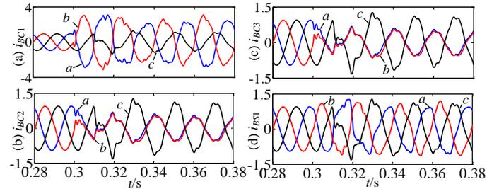
Fig. 8. Three phase currents flowing through circuit breakers during symmetrical fault F2: (a) cluster breaker  $B_{C1}$ , (b) cluster breaker  $B_{C2}$ , (c) cluster breaker  $B_{C3}$ , and (d) string breaker  $B_{S1}$ .
