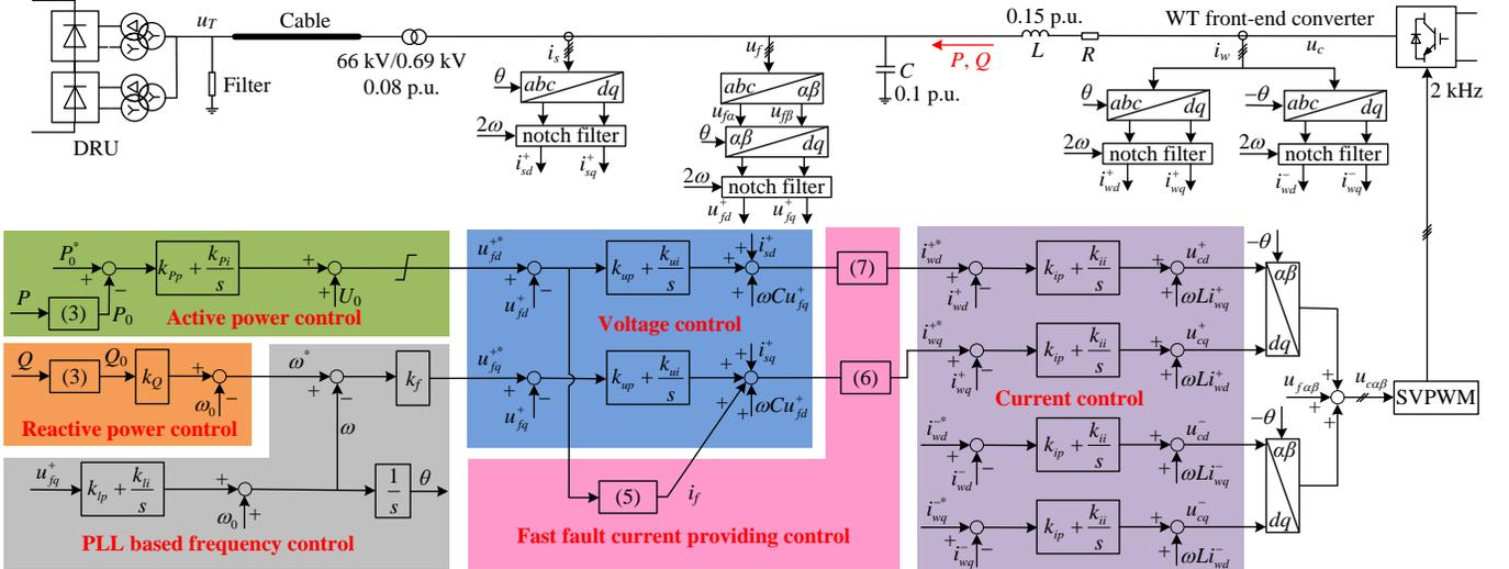
Fig. 2. Proposed control strategy of offshore WT front-end converters connected with DRU-HVDC.
