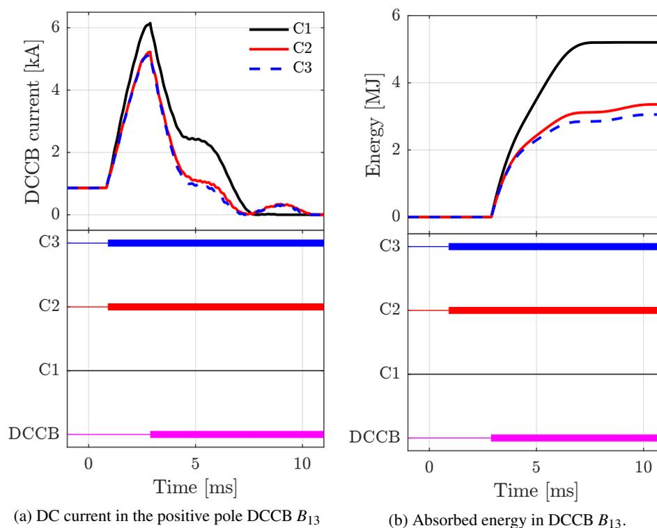
Fig. 5: Simulation results of the DC fault current and energy absorption in DCCB  $B_{13}$  of Fig. 4.
