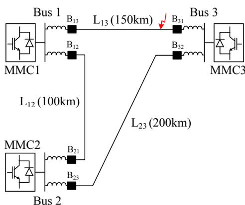
Fig. 4: HVDC grid test system.
