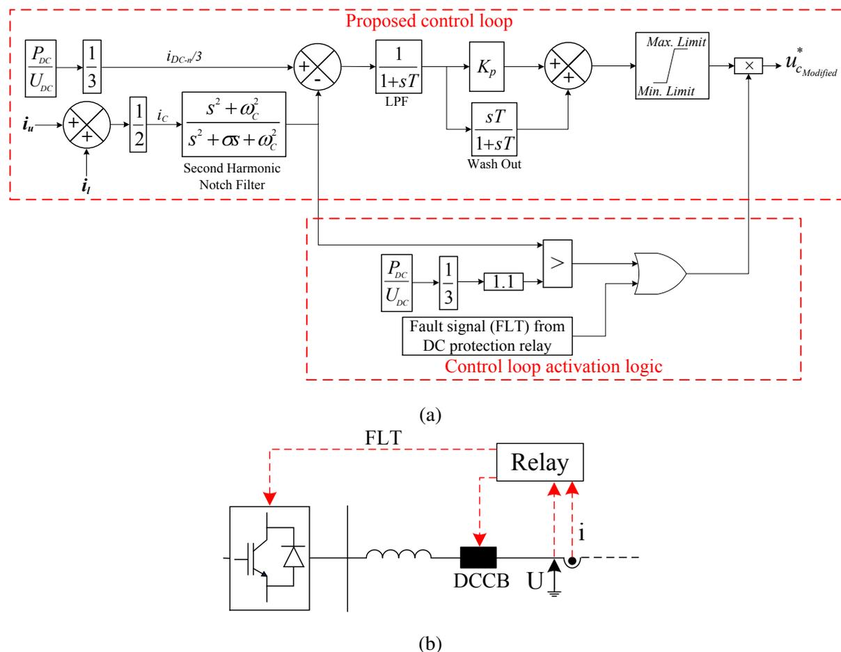
Fig. 2: (a) The structure of the proposed DC fault current signal reduction controller, (b) communicated signals between DC protection relay and converter station.
