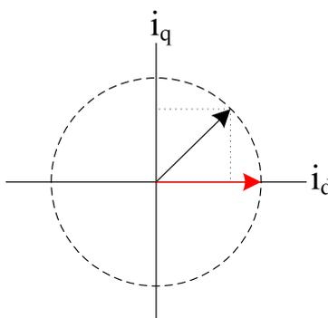
Fig. 3: Active current order margin extension of the MMC under DC fault.
