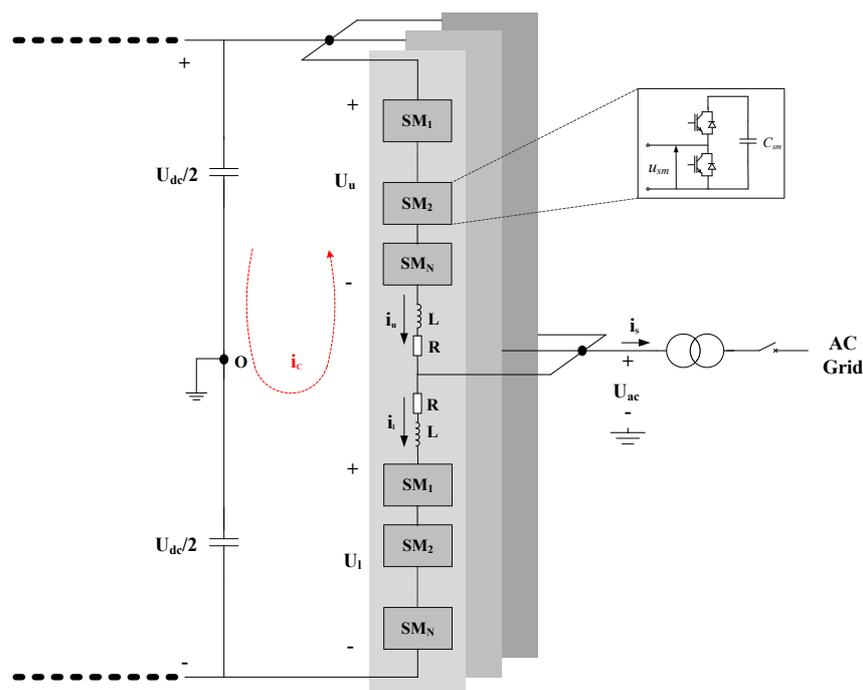
Fig. 1: Equivalent Circuit of the Half Bridge MMC
