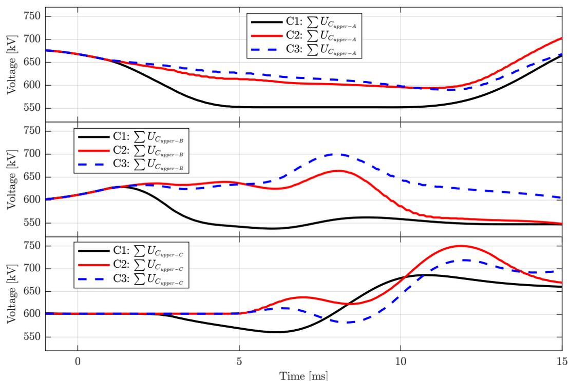
Fig. 6: The summation of submodules voltages of the upper arms of MMC1.
