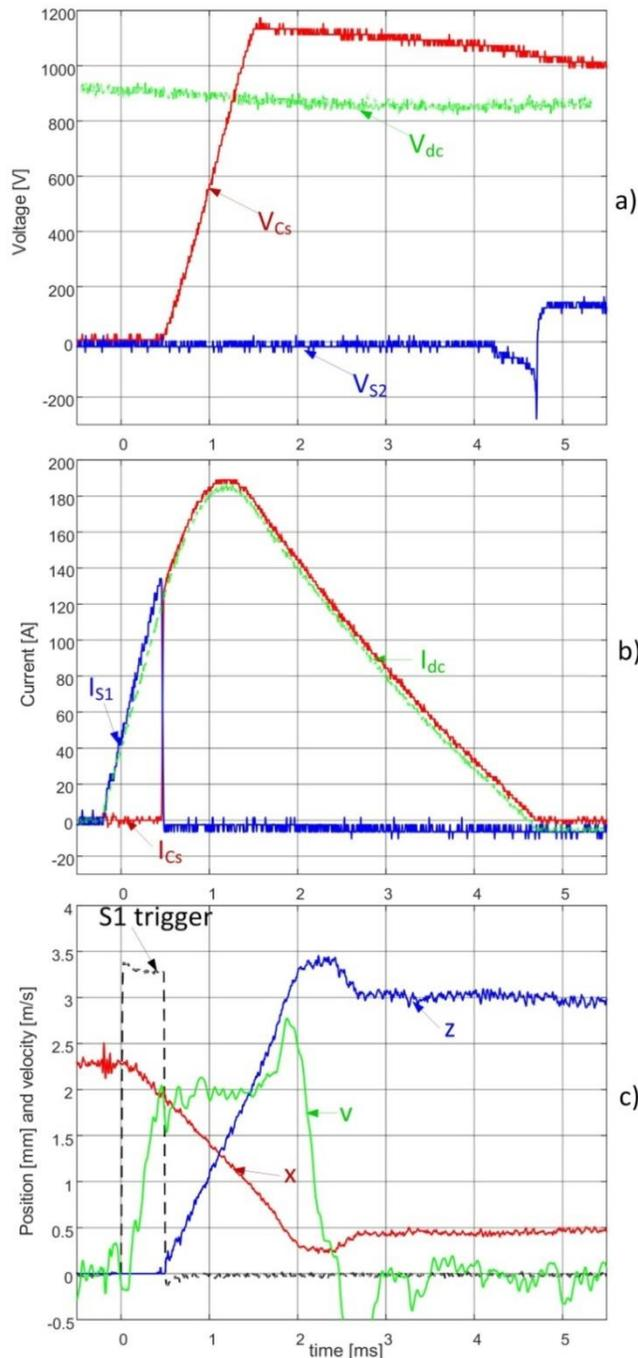
Fig.2. Experimental DC CB testing results. a) Voltages, b) currents, c) contact position and velocity.
