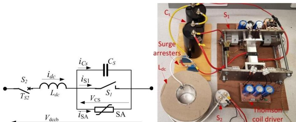
Fig.1: Schematic and experimental setup of LC DC Circuit Breaker.
