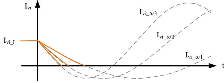
Figure 2: Influence of natural frequency on current-zero profile
