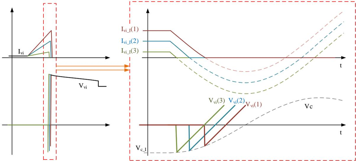
Figure 3: Influence of interrupted current on main interrupter initial TIV stress. Dashed lines represent the prospective current and voltage profiles if interruption does not occur
