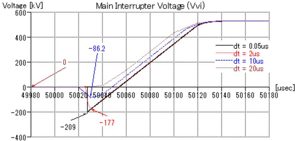
Figure 4: Simulation results of the initial transient interruption voltage across the main interrupter, performed with EMTP software. Simulation cases with various time-steps have been shown to illustrate the difficulty in accurately capturing the transient.
