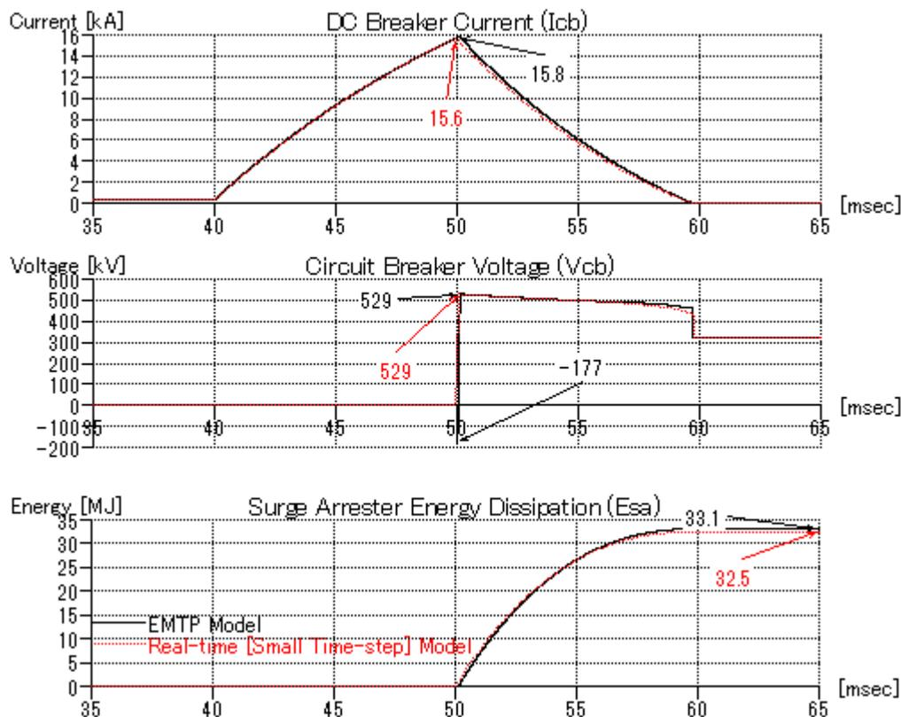
Figure 6: Comparison of Mechanical DC Circuit Breaker PSCAD and Small Time-step RTDS Model
