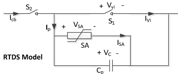
*Figure 5: Real-time Mechanical Circuit Breaker Model, implemented in both small and normal time-step..*
