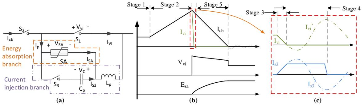
Figure 1: Mechanical circuit breaker topology and key waveforms during interruption. Dashed lines represent prospective currents (i.e. if no interruption occurred)
