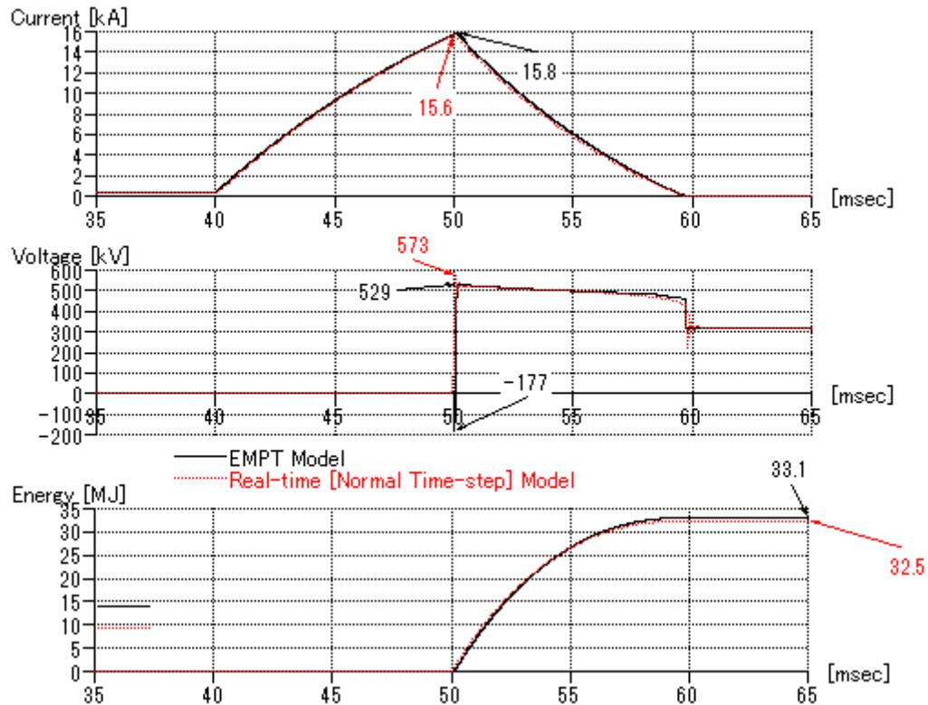
Figure 7: Comparison of Mechanical DC Circuit Breaker PSCAD and Normal Time-step RTDS models
